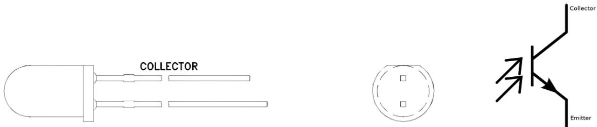
In the collision tutorial, we used a pull-down resistor to help us read the state of the switch. In this case we'll use a pull-up resistor. The voltage across the phototransistor will tell us if IR light is shining on it.
